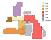
Diagram depicting the key phases of the construction of 'The Fry Building' from 1880 to 1936.
